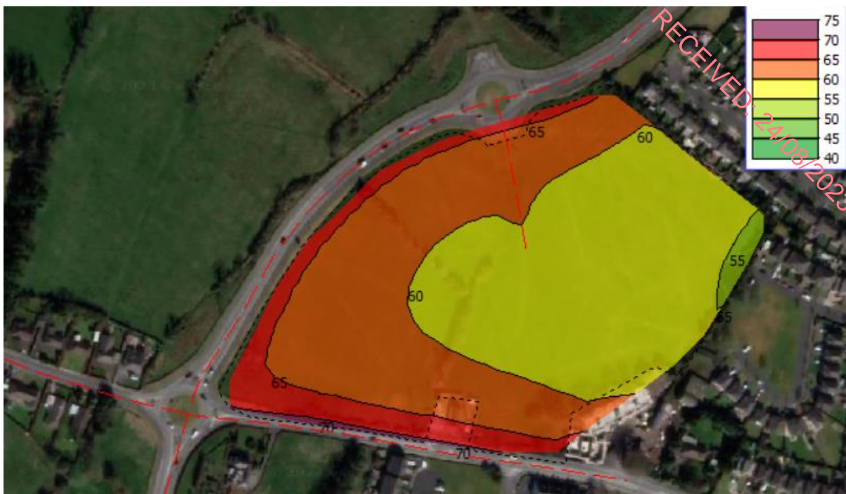
Figure 9.8 Daytime noise contours in dB(A) over existing site – in the absence of the development
